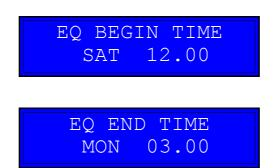
NOTE:(disabled change of minutes)NOTE:These parameters set a time window during the week in which the<br/>charger is allowed to fully charge and Equalize the battery.<br/>It's recommended to set a minimum Equalize time of 12 hours<br/>after the normal completion of the charge cycle.
